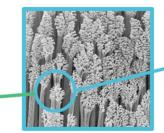
The unique geometry of our Dry Adhesive mimics the gecko's foot structure creating their signature noresidue grip. Our micro wedges replicate the soles of their feet that are covered in "hairs" called setae.
