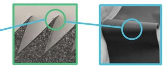
Each wedge tip, 1/100 of a human hair thickness, engage in shear using van der Waals force, not suction. A one square inch tile of our Dry Adhesive is covered in over 400 wedges that can hold 15 lbs. 6 tiles can pull a car !
